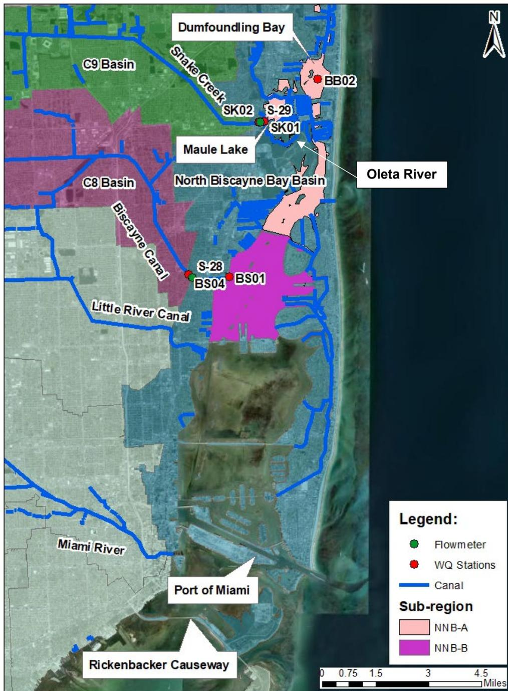
Figure 2-1: NNB -A and NNB -B in Relation to the WQ monitoring stations, Flowmeters, Canals, and Canal Basins
