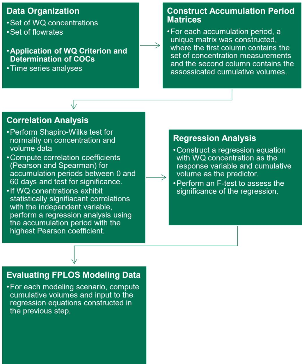
*Figure 4-1: Flowchart of Methods used for the Cumulative Volume Analysis*
